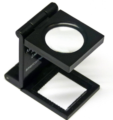
Figure 2. A loupe or a magnifying glass can be used to view the security microprint.
